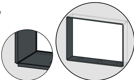
After applying the membrane as shown on the previous step, apply a generous amount of neutral-cure (non-acetic) silicone to the wall, along the sides of the wall support, and around the edges and sides of the recessed part of the niche to ensure a strong, watertight seal.
