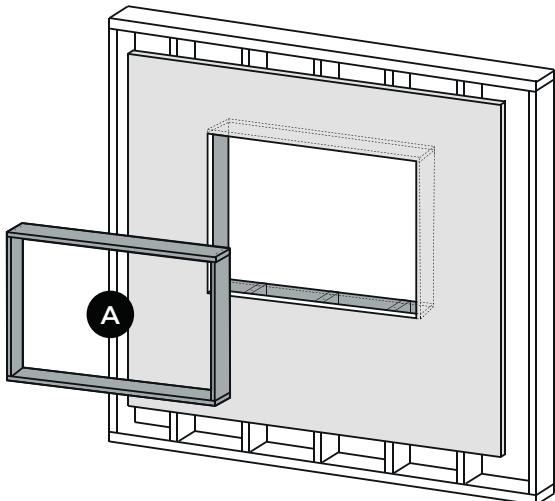
We recommend using a self-adhesive membrane on the inside of the frame, protruding 1/4 inch to waterproof the opening.
