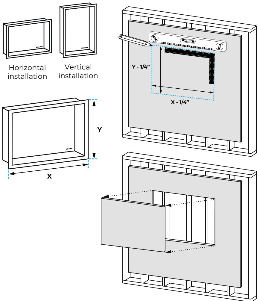
Build wall support all around the niche (A) in order to ensure proper support.
